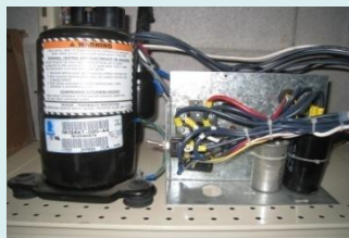
Like NEW Tecumseh Rotary compressor Model RKA5490EXA 115V R22 3/ 4 H.P. 9200 btu@45F w/electrics Made in USA $145
